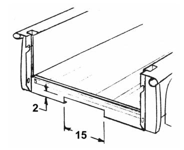
3. Temporarily clamp the pan side panels under the lower rear flanges of the bed sides so that the pan fits in position between the bedsides. The top of the pan should be tight against the rear sill. Check that the license box cut out allows clearance for the tag light socket and wiring. Also verify that the tailgate opens without binding against the pan. Adjust tailgate position if necessary.
