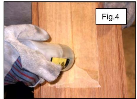
5. While the glue is still wet, flex the board in the area of the crack to encourage the glue to flow down into the crack. Use a thin strip of metal such as a feeler gage to push the glue into the crack if necessary. Be sure to pour more glue on the crack if it is not completely filled.
