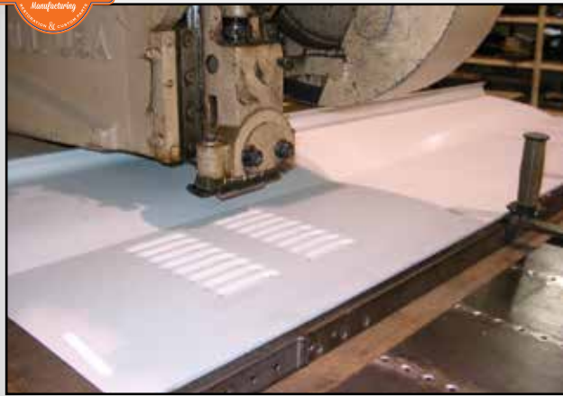
Louvres are punched in many of our MAR-K™ parts like rear pans and tailgate covers using this louvre press.
