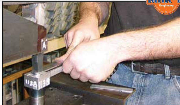
A MAR-K employee attaches the two link pieces to each other using this special pressing tool.
