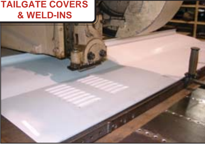
Louvres are punched in many of MAR-K parts like rear pans and tailgate covers using this louvre press.
