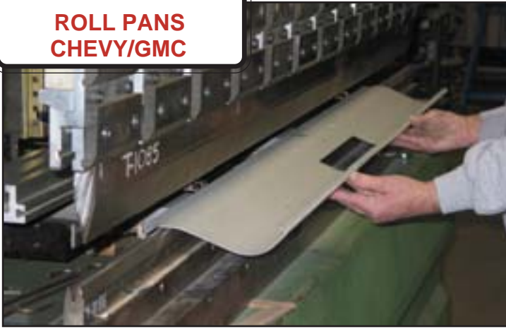
Rear Pans are formed in this press brake. Custom tools needed to make parts are designed and built at MAR-K.
