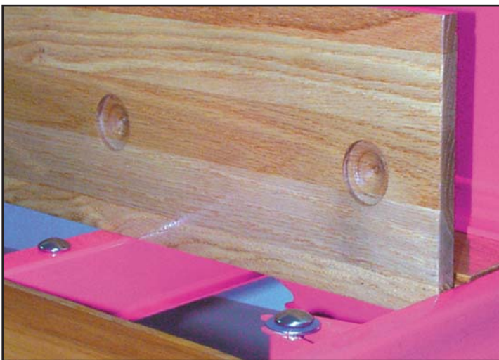
The bottom surface of the wood is drilled with a recessed clearance around the bolt head. The boards and strips rest on the cross sills as original, completely hiding the bed-to-frame and bed strip bolts.
