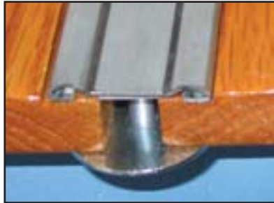
Polished stainless material is put into a roll former to make the bed strips with hidden fasteners.
