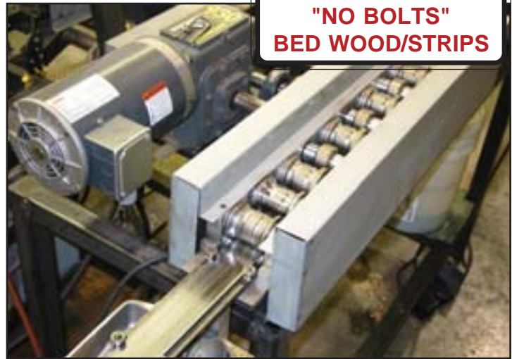
Polished stainless material is put into a roll former to make the bed strips with hidden fasteners.
