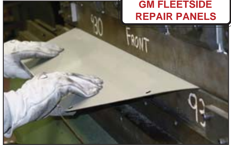
The top of MAR-K's Fleetside Repair Panels is embossed with an offset using this CNC press brake.
