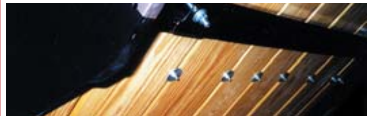
1972 GMC Stepside - William Thornton, Lenox, MA Shows how the bed strip bolts fall between the wood boards and bolt underneath the wood. Where there is not a cross sill, the bolts are secured by flat washers.
