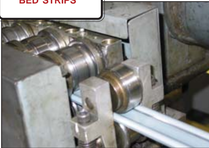
Steel material goes through a roll former to create new GM, Ford or Dodge bed strips.
