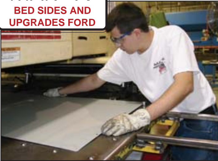
MAR-K bed sides begin with electro-galvanized steel punched in our CNC Turret punch press.
