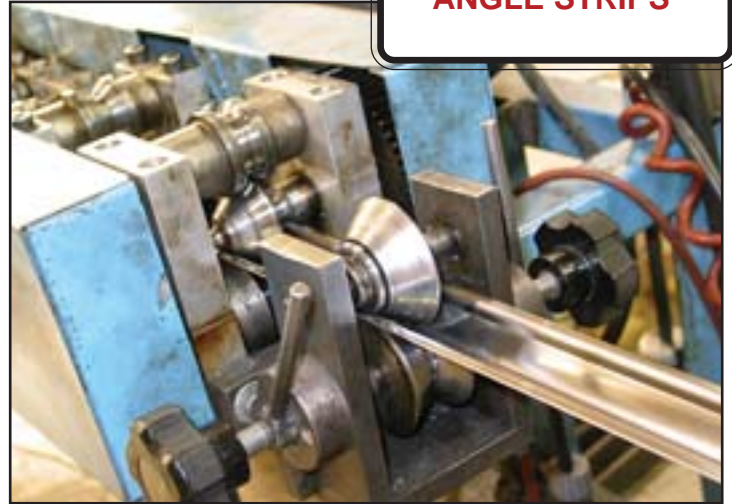
Polished stainless material goes through a special roll former to create the bend in angle strips.
