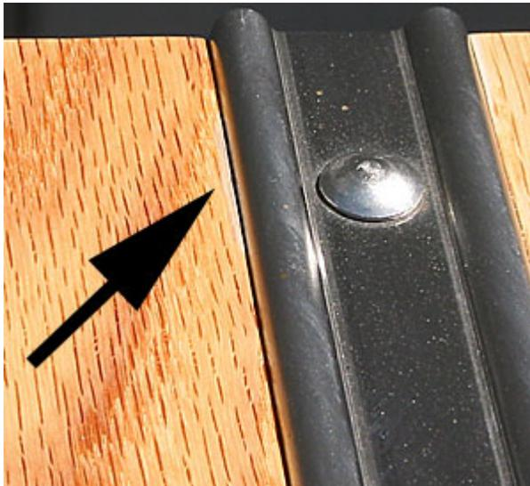
Sample number 3 is now showing a discoloration in a few spots, which is typical of the failures we have seen. This finish is RAKA epoxy with automotive clearcoat top coat. The failure is just beginning to show. We will provide more information in future updates as this finish continues to deteriorate.
