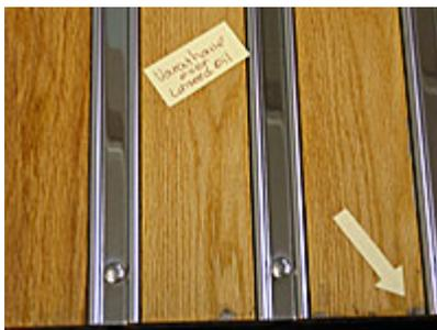
Varathane exterior gloss urethane. The samples which were sealed with linseed oil first lasted much better than the samples which were applied directly over bare wood. This product was not as durable as Minwax or McCluskey's in our tests. We have decided not to continue testing the Varathane product.
