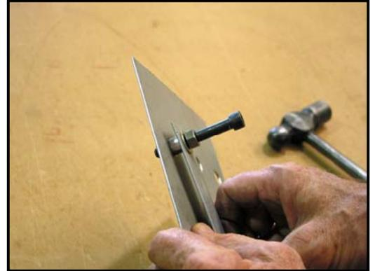
8. For this step, you may need a helper. Use a wrench to keep the bolt head from turning and hold the scrap piece of metal. With another wrench, start to back the hex nut off of the bolt. The hex nut will draw the bolt outward while compressing the insert behind the sheet metal panel.
