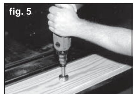
6. From the top surface, drill through the 1/8" pilot holes with a 1/2" drill bit to complete the bed-to-frame holes. See figure 6. Before drilling the 1/2" hole, place a piece of scrap wood directly under the 1/8" hole to prevent splintering as the drill breaks through.
