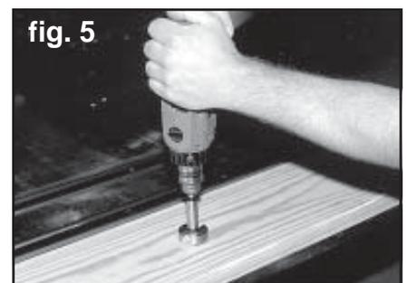
6. From the top surface, drill through the 1/8" pilot holes with a 15/16" wood bit to complete the bed-to-frame holes. See figure 6. Before drilling the 15/16" hole, place a piece of scrap wood directly under the 1/8" hole to prevent splintering as the drill breaks through.
