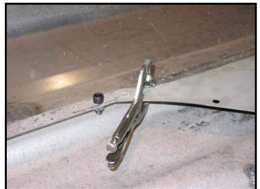
11. The rear of the patch panel has a lower flange hole that matches up the rear stake pocket. Use a 5/16" diameter carriage bolt and bolt these two panels together.
