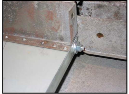
There are many methods of attaching panels such as these. We have chosen to plug weld the overlap seam. In order to do this properly, the two pieces of metal must fit tightly against each other. The following is one method of accomplishing this.
