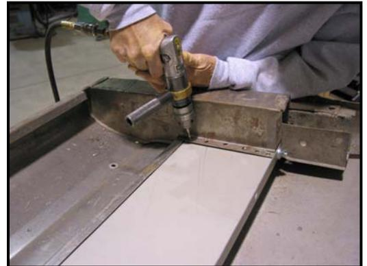
17. Place a sheet metal screw into these locations. This process makes sure that the metal pieces are tight against each other before the plug welding begins and ensures good penetration of the weld.
