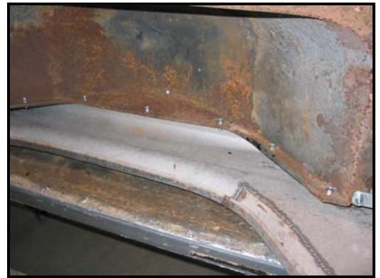
19. With the wheelhouse installed, remove one sheet metal screw at a time and plug weld the hole. You may start at the front or rear panel, vertical or horizontal seams. Make sure you are getting good penetrating plug welds.
