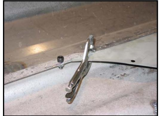
13. Approximately 3" away from the 3/8" diameter bolt, center-punch the seam.
