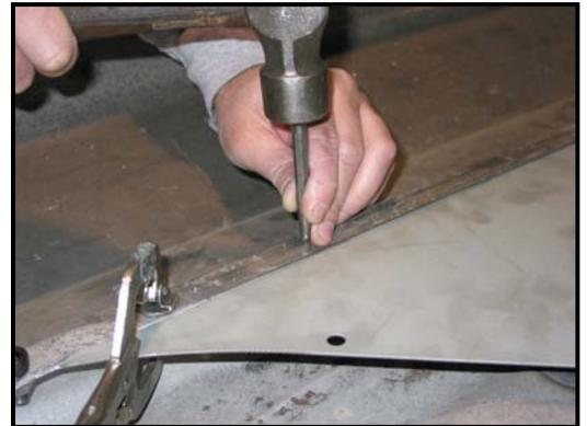
14. Drill this mark with a #24 or 5/32" drill bit through both panels. Drill through the same hole again with a slightly larger drill but this time only through the top layer. Thread a #10 x 1/2" sheet metal screw into both panels. The larger hole on top will allow the screw to spin while the smaller 5/32" hole in the patch panel will grab the screw. Use caution to be sure that no chips are pushed into the seam between the patch panel and the bedside.
