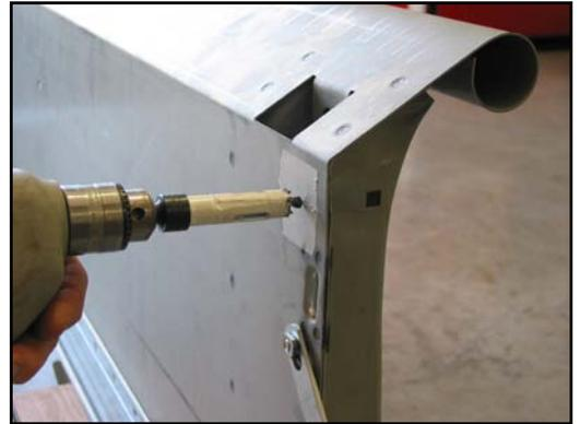
19. Remove the burr from the holes and install the supplied rubber grommets.
