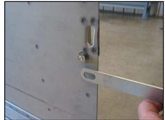
11. Lower the tailgate to the open position. Close the tailgate slowly making sure that the links fold downward this time. The links should fold smoothly into the tailgate end as the tailgate is raised. The tailgate should move to the fully closed position without causing any binding in the link assemblies.
