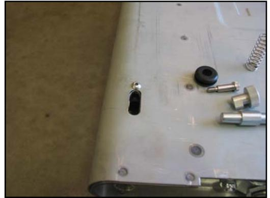
14. The latch plunger and the latch barrel need to match. The latch plunger and the barrel have an angled cut on them that controls the direction of the locking knob. The angle on these needs to be pointing the same direction as shown. Slide a spring onto the latch plunger and slide the assembly into the latch barrel.
