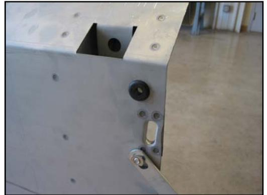
20. Close the tailgate and release both latches. Make sure that they enter the grommets.
