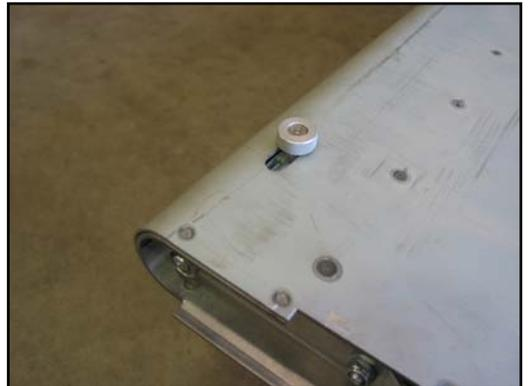
17. We need to drill a hole in the bed side for the latch to fit through. Raise the tailgate and observe where the latch plungers will contact the bed sides. Place masking tape on the inside area of the bed side where the latch plunger will hit. Release the plungers by turning the aluminum knobs. The plungers have a point on them that will mark the tape.
