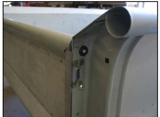
You have now successfully installed your new tailgate, hidden latch system, and the link assemblies. During final assembly, use a quality lubricant on all the moving parts and a thread locking compound on the assembly hardware.
