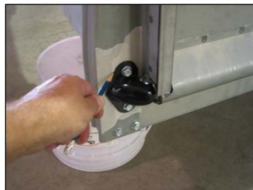
4. Remove one hinge and remove the tailgate. Install the hinge back in the same location so that both hinges are in the exact mounting position they were when the tailgate was installed and properly aligned.
