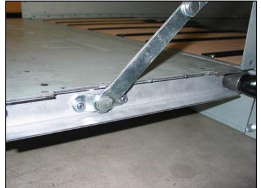
10. Carefully raise the tailgate while folding the links in the upward direction. This will allow the slot in the link assembly to fit onto the fixed pivot that you bolted to the bed side.
