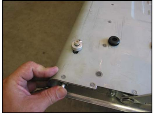
16. Pull the knob towards the center of the tailgate and twist to lock it into position. You may need to twist up or down depending on which latch barrel and plunger you put in. You may also switch these from end to end on the tailgate to reverse this direction.
