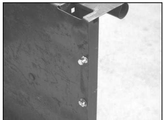
10. Re-attach the tailgate using the masking tape mark for the hinge location reference. Support the tailgate in the horizontal or open position.
