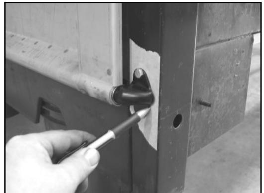
4. Remove the hinge marked in step # 3 above and remove the tailgate. Install the hinge back into position using the marked masking tape as a guide.
