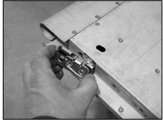
12. Each latch is held to the tailgate with (2) metric M6-1.0 x 30 mm Phillips flat head screws provided in the kit. You should be able to see the actuating arm and nut through the slotted hole in the tailgate skin.
