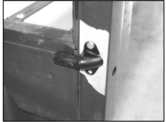
5. Slide the template provided onto the hinge far enough that the template can lie flat against the inside of the bedside. The outer edge of the template should be even with the outer edge of the bedside. Clamp the template in place.
