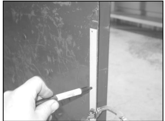
7. Remove the template and center punch these locations and drill 5/16" holes through the bedside. Remove the burr from both holes on the inside and outside. Repeat steps #5 through #7 for both bed sides.
