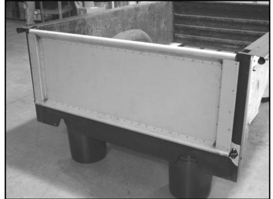
2. Place some masking tape over the hinge attaching locations on one of the bedsides. Install the hinges and the new tailgate and make sure it is aligned to your satisfaction.
