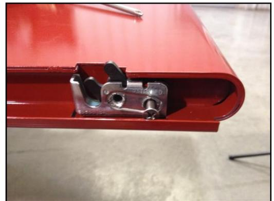
16. Install the other flat head screw into the latch and tighten both with a Phillips screw driver. Repeat steps #14-#16 for the other side.
