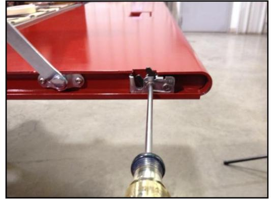
17. Push down on the latches to close them. You should hear two distinct clicks as they latch shut. Pull up on the handle. Both latches should release approximately the same time.
