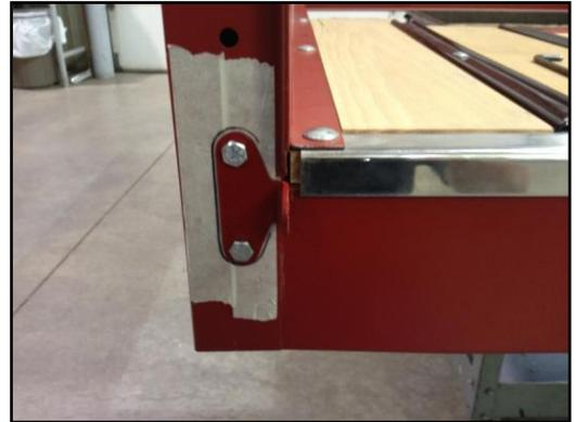
6. Bolt the template provided onto the hinge with the 5/16-18 x 1/2" button head screw and flat washer and nut provided so that the template can lay flat against the inside of the bedside. The outer edge of the template should be even with the outer edge of the bedside. Clamp the template in place.
