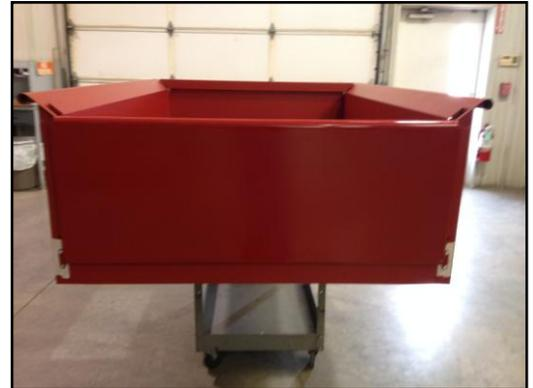
2. Assemble the tailgate hinge trunnion to the hinges as shown with the  $5/16-18 \times 1/2$ " button head screws. Tighten the screws with a  $3/16$ " allen wrench.
