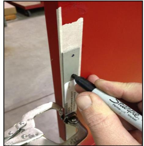
8. Remove the template and center punch these locations and drill 5/16" holes through the bedside. Remove the burr from both holes on the inside and outside. Repeat steps 5 through 8 for both bed sides.
