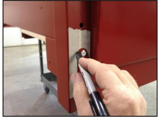
5. Remove the hinges marked in step # 4 above and remove the tailgate. Install the hinges back into position using the marked masking tape as a guide. Also remove the trunnions from the hinges.
