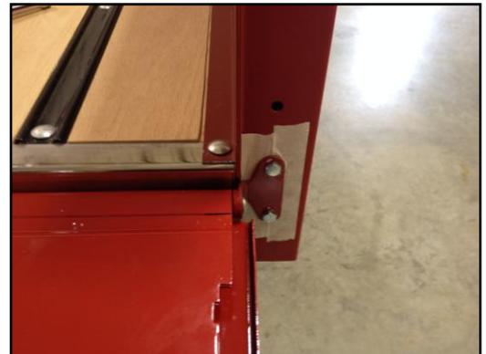
4. Mark the location of the hinges onto the masking tape so that they may be removed and re-installed in the same exact location.
