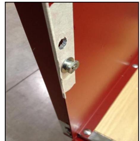
10. Re-attach the trunnions to the hinges and re-attach the tailgate using the masking tape mark for the hinge location reference. Support the tailgate in the horizontal or open position.
