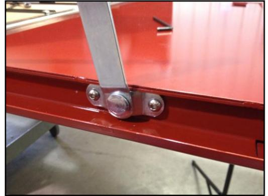
12. Lift the tailgate while directing the link assembly arms to the pivots attached to the bedsides. The link assembly arms will need to be folded in the upward direction for this. Lift the assembly until the slot in the link will fit onto the pivot.
