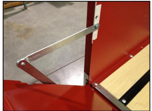
13. Attach a striker to both bedsides in the top holes as shown. Use the 5/16-18 x 1/2" button head screws on the outside of the bedsides. Tighten the strikers with a 9/16" wrench while holding the button heads with a 3/16" allen wrench.
