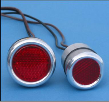
This is an accessory light and is to be electrically connected to your existing light system. The bulb is a 12 volt, type 194 miniature single filament bulb commonly used in GM side marker applications. The lighted hole cap will provide additional lighting at the rear of your truck, but is not intended to replace your DOT legal taillight/brake light system.
