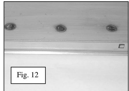
7. Grind the plug welds smooth and prepare for painting. See figure 13.
