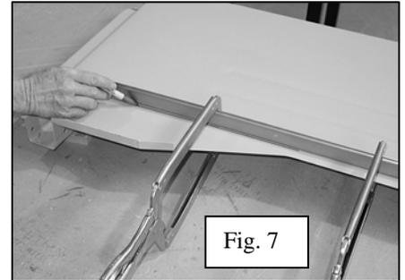
2. Remove the angle and draw a line the length of the bedside at the position of the plug welds, about 3/8" above the bottom of the angle strip. The welds should be midway between the bottom leg of the angle and the rolled edge of the top of the angle. See figure 8.
