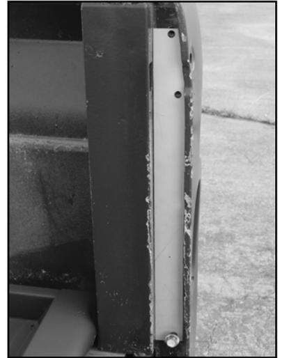
5. We need to drill the holes out to  $17/32$ " in order to fit the nutserts supplied in the kit. Mar-K has a drill bit available for this. (See part # 50622 online).
