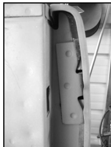
3. After the bracket is removed, clean up this area with a wire brush. There will likely be corrosion behind this bracket. Your bed side should now look like this. The two holes in the middle and the large rectangular hole will not be used. These holes will be covered by the new brackets from the other kits. They can be left open or welded shut.
