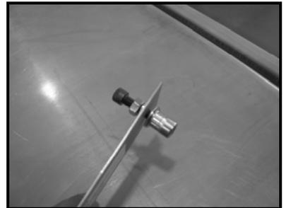
8. Place the insert into the hole in the bed side. Make sure to hold the insert flange tight against the bed side. Allow the template to rotate downward to the hinge area of the tailgate. This template will act as a handle to keep the insert from rotating when the nut is tightened.
