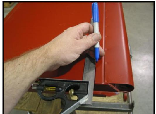
4. Measure towards the bottom of the tailgate from this line 2-5/8" and make another mark. Make a 1-7/8" line on this mark as before. Join the ends of these two lines to create a rectangle
