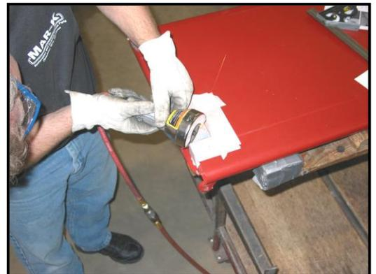
9. When you reach the bottom of the two vertical lines, Turn your tool back to flat but tilt it as shown. We need to cut along the bottom of the vertical sheet metal that is left. You will be leaving the strip of metal at the base that is spot-welded to the outside skin of the tailgate.
