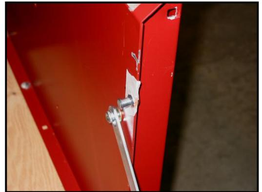
30. Pull up on both black knobs to release the latches. Slowly close the tailgate and watch for the strikers to enter the latch area. Continue closing the tailgate until each latch makes two clicking noises. If the latches do not close on the strikers properly, loosen the strikers and adjust their position until they do.
