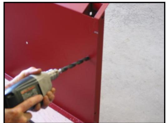
21. Test fit the threaded insert into the 17/32" diameter hole. Use a round file to enlarge the hole if the insert will not fit. Often, a drill will not make a perfectly round hole in sheet metal. Use the file to make the hole round. The insert must be installed so that its' flange is against the sheet metal surface of the bed side.
