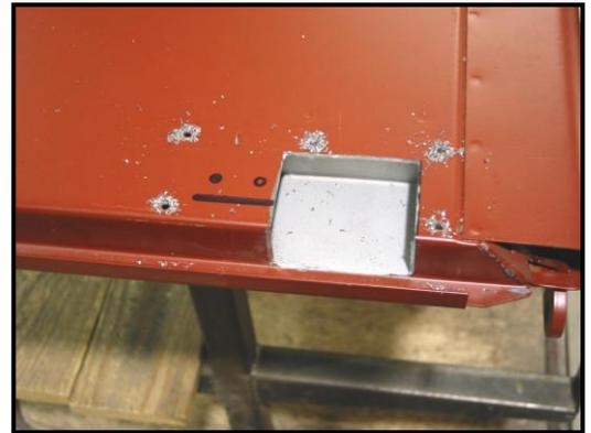
15. Center-punch the two larger marks and drill these with a 9/32" diameter drill. Center-punch the two ends of the area that will be slotted and drill these with a 7/32" drill. Cut the area of the slot out with a rotary tool with a reinforced cutting wheel. Place some masking tape along the edges between the holes to guide you. You can do this cutting with the high speed 3" tool, but you will have greater control with the smaller device.
