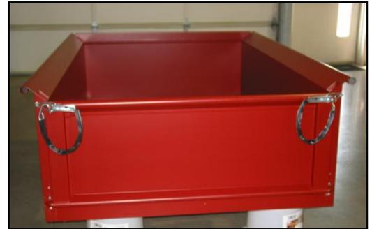
3. Support the tailgate in the horizontal (open) position. The tailgate has been removed in the photograph, but this is not necessary. Measure up from the bottom curl of the tailgate (15-1/2" for a 53-72 short bed) or (17-1/4" for a 73-87 short bed and 53-72 long bed) and make a mark. Using a combination square, draw or scribe a line 1-7/8" long inward towards the center of the tailgate.
