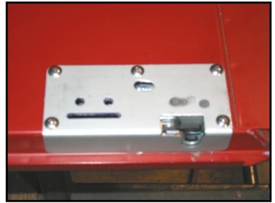
17. Slide the link assembly through the slot in the adapter panel and tailgate skin. Attach the link assembly to the tailgate with two 1/4-20 x 1/2" button head screws. Tighten the screws with a 5/32" Allen wrench. **Note: It is important to notice that there is a left and right link assembly due to the pivot bracket of the link assembly. The offset part of the bracket where the rivet is should be at the bottom towards the tailgate hinge. This is the left (driver) side link shown installed.**
