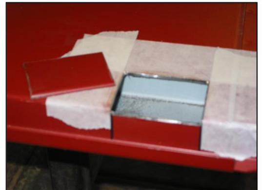
8. Cutting the vertical section of material away is a little harder. Rotate the cutting tool at an angle and move into the opening until you can cut all the way to the bottom of the vertical wall. The object here is to cut the vertical section without cutting through the outside flange of the tailgate. This outside flange is seen when the tailgate is closed and is not covered up by the adapter panel.
