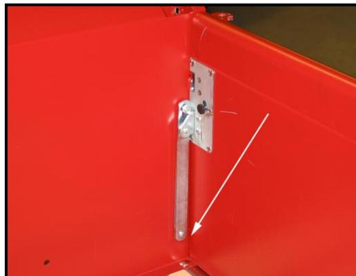
27. The latch striker is the only thing left to do. With the tailgate in the proper closed position, make a mark on the bed just at the top of the opening of the latch area on the adapter panel as shown. The latch striker will be positioned 3/8" lower from this mark. It will need to be 3/8" from the back edge of the bed side.
