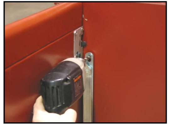
20. Lower and support the tailgate once again. Measure in from the back edge of the bed side 1-9/16" at the same vertical position as the drill mark and make a mark. Center-punch this position. Drill this position on each bedside with a 1/4" drill bit. Now drill this hole to a final size of 17/32".
