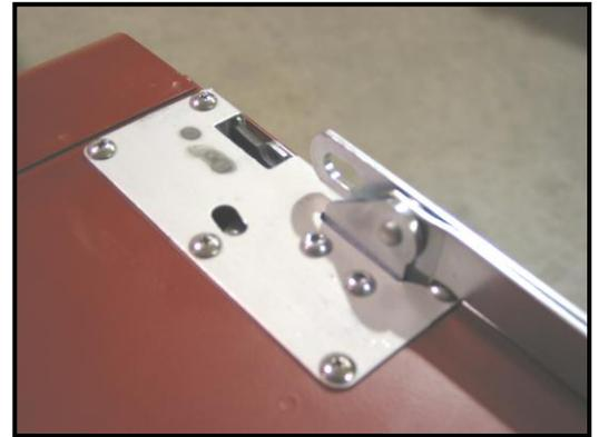
18. Thread the aluminum spacers completely onto the black knobs. Thread the knobs into the rotary latches through the slotted hole in the adapter panels. Check the operation of the latch. Lift up towards the top of the tailgate until the latch releases.
