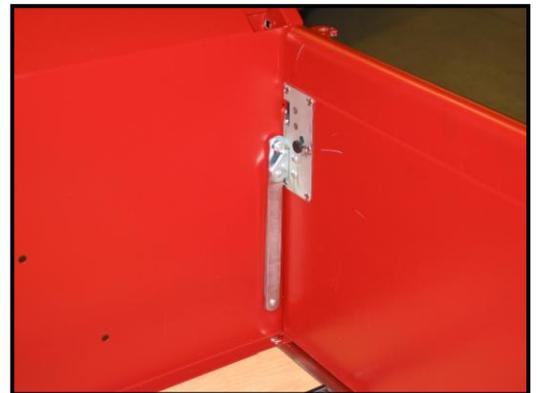
You have successfully installed the hidden latch and link assemblies. At final assembly, use a thread locking compound on all threaded areas to prevent them from coming loose.
