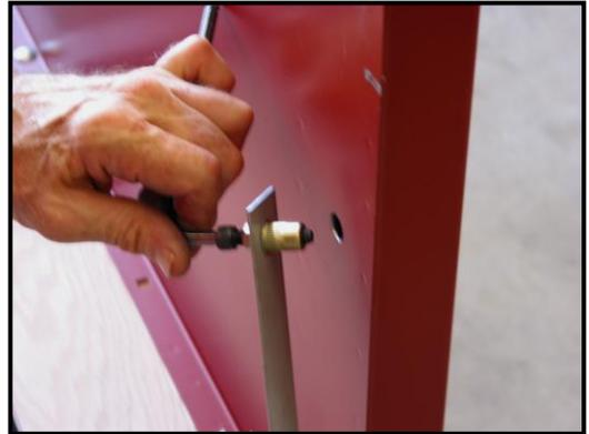
23. Place the insert into the hole in the bed side. Make sure to hold the insert flange tight against the bed side. The sheet metal scrap will act as a handle to keep the insert from rotating when the nut is tightened.
