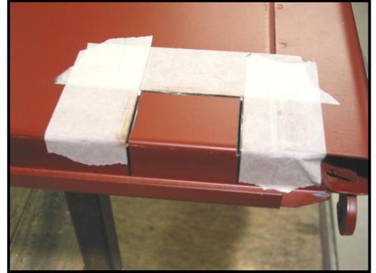
7. Cut horizontally between the cuts in the previous step until this piece is removed completely.
