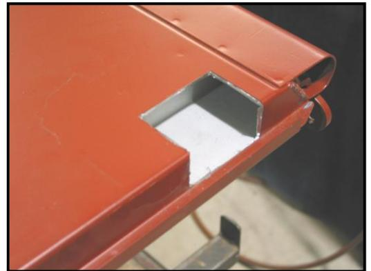
10. Remove the burs left by the cut-off wheel from the opening. Also make sure that the measurements are good. Refer back to step #3 & 4. Fit the adapter panel into the opening and check for clearance. **The bottom of the adapter panel should be 10-11/16" from the bottom of the tailgate.**
