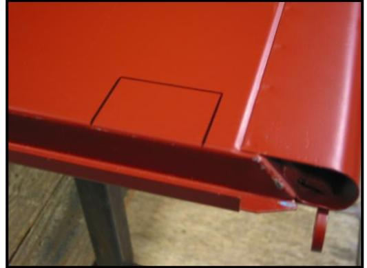
5. Create a vertical line on the edge of the tailgate from both horizontal lines. This marked area will need to be removed to allow the hidden latch to fit into the inside of the double wall structure of the tailgate.
