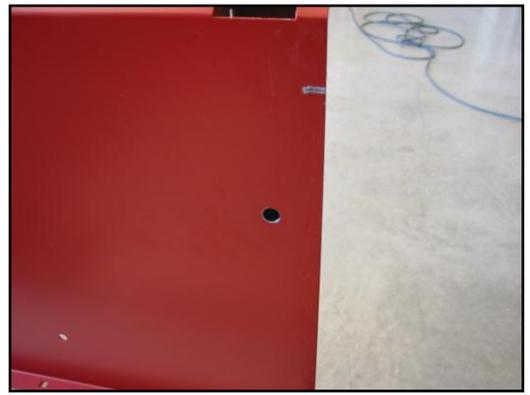
22. Special tools are available to squeeze the threaded inserts but we will show you how to do this without these special tools. Obtain the 5/16"-18 x 1-1/2" bolt and 5/16 hex nut supplied in the kit. Thread the hex nut about 1" onto the bolt. Place the bolt through the supplied flat washer. Use a scrap piece of sheet metal with a 3/8" hole and place it on the bolt after the washer. Next thread the insert onto the bolt with the flange of the insert towards the sheet metal finger tight.
