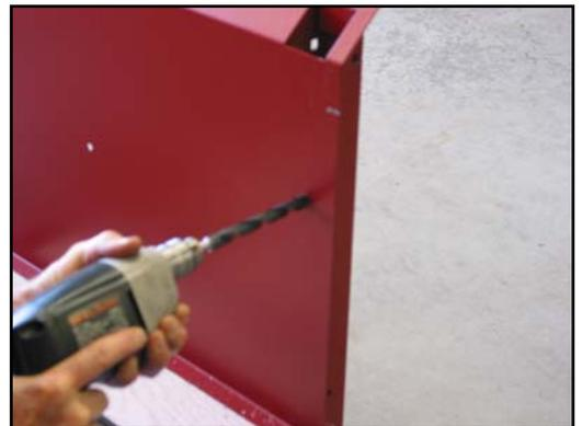
12. Test fit the threaded insert into the 17/32" diameter hole. Use a round file to enlarge the hole if the insert will not fit. Often, a drill will not make a perfectly round hole in sheet metal. Use the file to make the hole round. The insert must be installed so that its' flange is against the sheet metal surface of the bed side.
