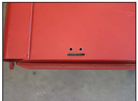
9. Insert the link assembly into the slotted hole. Attach the link assembly to the tailgate with two 1/4-20 x 3/8" button head screws. Tighten the screws with a 5/32" Allen wrench. It is important to notice that there is a left and right link assembly due to the pivot bracket of the link assembly. The offset part of the bracket where the rivet is should be at the bottom. This is the passenger side link shown installed.
