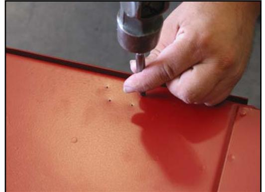
6. Drill the outer-most holes on each end with a 3/16" diameter drill. Drill the two inner-most holes on each end of the tailgate with a 1/4" drill. Be careful to not damage the outer side of the tailgate with the drill point. You may choose to use a drill stop on the drill bit or wrap some masking tape on the bit to stop the drill from hitting the outside of the tailgate skin. Repeat for opposite end of the tailgate.
