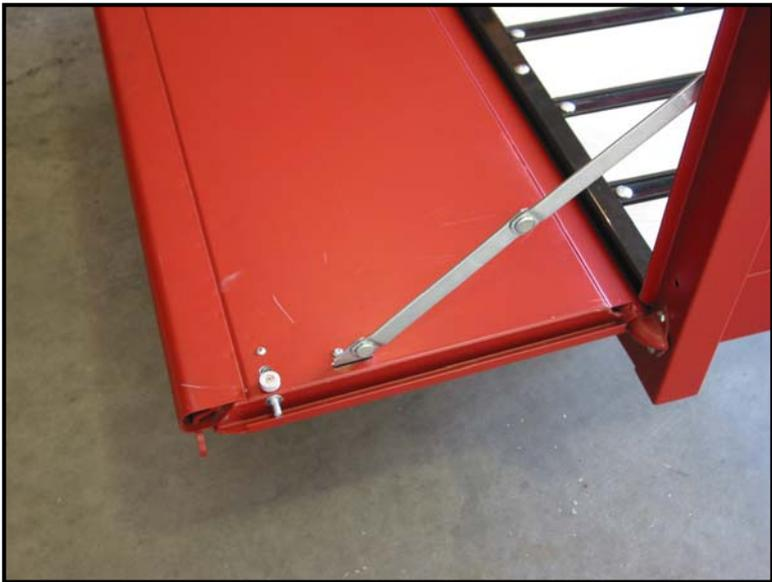
You have successfully installed the link assemblies. At final assembly, use a thread locking compound on all threaded areas to prevent them from coming loose. This kit is greatly complimented with our hidden tailgate latch which is Part # 102884 shown already installed.
