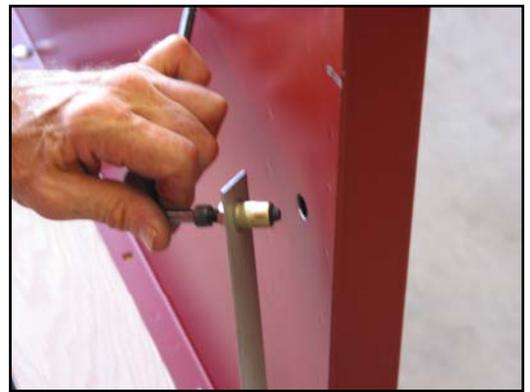
14. Place the insert into the hole in the bed side. Make sure to hold the insert flange tight against the bed side. Allow the template to rotate downward to the hinge area of the tailgate. This template will act as a handle to keep the insert from rotating when the nut is tightened.
