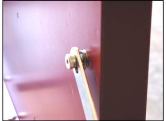
17. Raise the tailgate slowly to the closed position. The links should fold smoothly downward while closing. Supplied in the kit are two self-adhesive bumpers. Attach these bumpers where the link assembly will contact the tailgate when closed.
