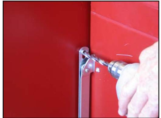
11. Lower and support the tailgate once again. Measure in from the back edge of the bed side 1-9/16" at the same vertical position as the drill mark and make a mark. Center-punch this position. Drill this position on each bedside with a 1/4" drill bit. Now drill this hole to a final size of 17/32".
