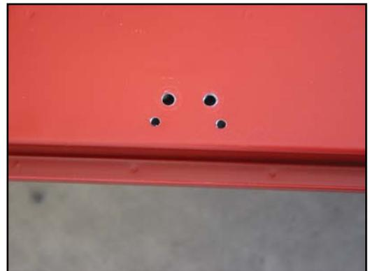
7. You need to cut a slot for the link assembly mounting bracket to fit through. Place masking tape on each side of the 3/16" diameter holes as shown. This will make it easier to see where to cut. Do both ends of the tailgate.
