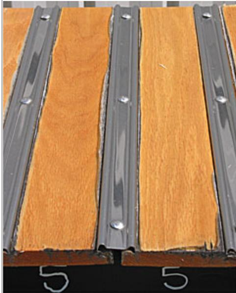
5. Oak boards, coated with two brushed coats of RAKA epoxy, cured one month, block sanded, and topcoated with three sprayed coats of Minwax Helmsman Spar Urethane.
