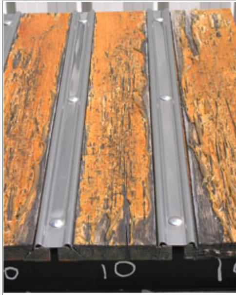
10. Oak boards, saturated with several coats of heated linseed oil until it would not absorb any more, cured three months, wiped with turpentine to remove excess dried linseed oil from the surface, and when dry, sprayed with three coats of Minwax Helmsman Spar Urethane.
