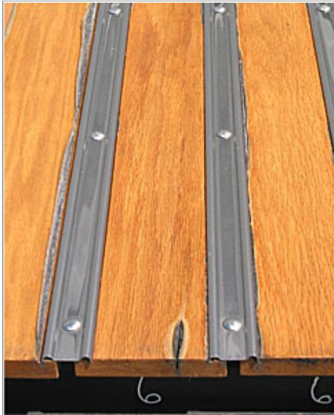
6. Oak boards, coated with three brushed coats of Pelucid three hours apart, cured 4 days, block sanded, and sprayed with three coats of Minwax Helmsman Spar Urethane.
