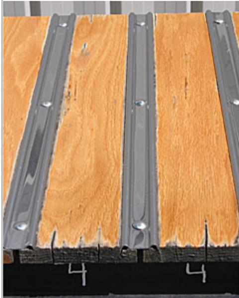
4. Oak boards, coated with one brushed heavy coat of CPES epoxy and three sprayed coats of automotive clearcoat. The clearcoat product was applied before the CPES was fully cured for best adhesion as recommended by the epoxy manufacturer, Smith & Co.
