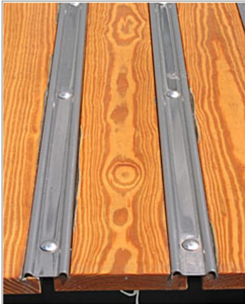
9. Pine boards, coated with three brushed coats of Pelucid three hours apart, cured 4 days, block sanded, and sprayed with three coats of Minwax Helmsman Spar Urethane.
