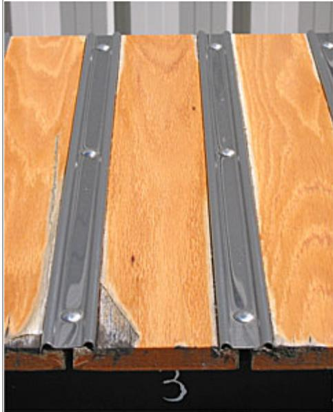
3. Oak boards, coated with two coats of RAKA epoxy, cured one month, block sanded, and topcoated with three coats of automotive clearcoat.
