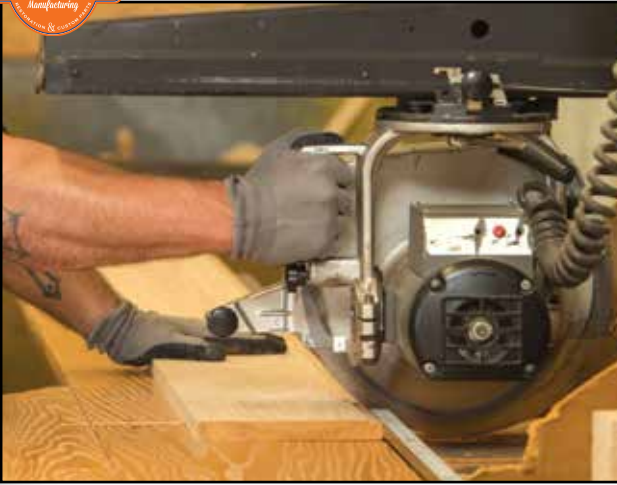
Cutting Bed Wood Boards in MAR-K's Wood Room. MAR-K grooves and cuts the boards to size.
