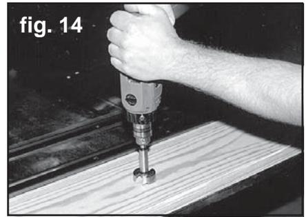
23. From the top surface, drill through the 1/8" pilot holes with a 1/2" drill bit to complete the bed-to-frame holes. See figure 15.
