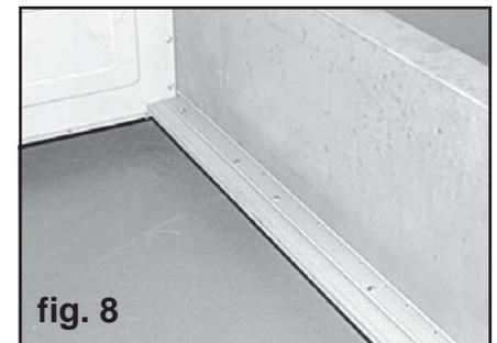
12. Attach the cross sills to the 5/16" angle strip bolts approximately **2-1/2"**, **26-11/16"** and **53-11/16"** respectively from the front bed panel. The cross sills should be installed so that when the bed is installed on the frame the cross sills should be open toward the ground. See figure 9. Install the lock washers and nuts hand tight.
