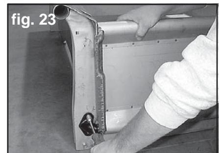
34. Attach one hinge onto passenger bed side rear stake pocket. Secure with (2) 5/16"-18 x 3/4" indented hex head bolts. Install tailgate to this hinge. Install second hinge into other end of tailgate. Bolt second hinge to driver stake pocket. See figure 23.
