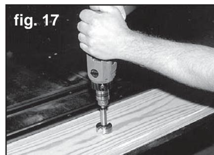
23. Using a 1-9/16" diameter Forstner bit, a drill press if available, or a hand drill, countersink each location approximately 1/8" to 5/32" deep. See figure 17.
