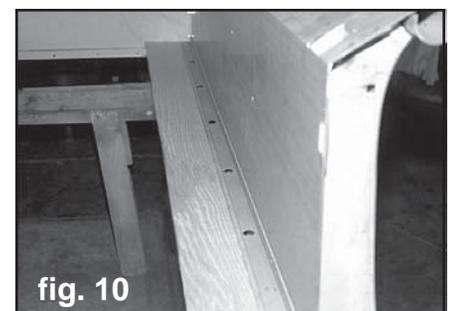
15. Attach the cross sills with brackets to the 5/16" bolts in the angle strips approximately **2-5/8"**, **26-5/8"** and **52-7/8"** respectively from the front bed panel. The two offset brackets go with the third cross sill from the front and the hole is offset toward the bed sides. Install lock washer and nut and hand tighten. The cross sills should be installed so that when the bed is installed on the frame the cross sills should be open toward the ground. See figure 11.
