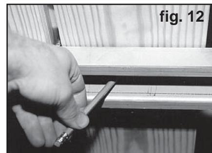
17. The second bed-to-frame bolt location is in the third cross sill counting back from the front bed panel. Mark the bottom of the wood boards through the 1/2" diameter cross sill holes that are **44-3/8"** apart from center of hole to center of hole. The second cross sill from the front bed panel does not have a bed-to-frame bolt.
