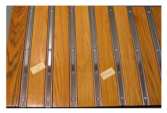
At this time, all the finishes have failed to at least some degree. We will conduct another test beginning about February 2005, using the coating systems that performed the best and adding other promising finish systems. Following are some notes regarding the performance of each coating.
