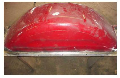
The repair flange should now be an integral part of the wheel tub. Sand these areas; primer and paint as desired.
