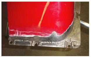
These instructions cover the repair of the wheel tub flange where it meets the wood floor in 1958 to 1966 GM trucks with the Fleetside bed. These areas are prone to rusting because of the wood holding moisture and the steel flange resting on the wood floor. This repair flange may be used to completely replace this flange or be used in pieces to repair this area. The wheel tub pictured at the left is an extreme case of deterioration caused by rust.
