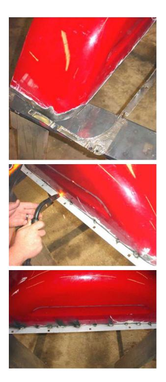
4. Fit the repair flange to the wheel tub. You may need to dress up the wheel tub where the damaged flange was removed. When the fit is good, tack weld the repair flange to the wheel tub in several places.
