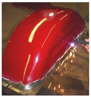
3. Remove the repair flange. Using a plasma cutter or a cut-off wheel, remove the damaged area of the wheel tub flange. Cut on the scrap side of the scribe line or marks made in the previous step. This wheel tub was rusted enough to need the complete flange replaced.
