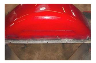
7. Grind the welds smooth on both top and the underside of the wheel tub. Work slowly and avoid building up too much heat. Be extra careful around the hump areas where the bed strips go. A grinder could easily damage this area.
