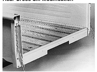
The installation of a MAR-K steel rear pan with a license indention usually requires modification to the rear cross sill. Since the "tag box" is indented, a space will need to be cut in the rear cross sill for clearance. The rear pan will not fit properly unless this is done.
