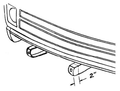
separating the baffle and grille, and sliding the upper flange of the pan between the grille and baffle. Holes must be drilled in the pan so that the original bolts will sandwich the pan mounting flange between the grille and baffle. The pan may be welded to the lower grille section at the installers option.
