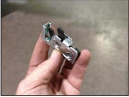
15. Place a flat head Phillips screw, provided in the latch kit, into the top hole of the latch. Slide the latch into position with the latch tilted slightly outward until lined up with the holes. Be careful to not move the shim. Tilt the latch toward the tailgate until it seats into position. It may help to slightly raise the handle in the tailgate which rotates the actuating arm.
