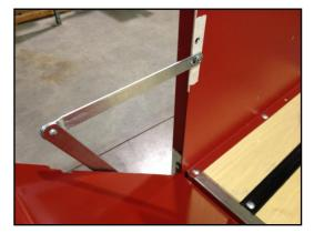
14. Place a shim into the latch area of the tailgate. Release the latch by rotating the inner black lever.
