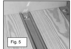
Insert the 5/16"-18 x 1-1/2" carriage bolts through all holes in 16. the bed strips. A few of the bolts will not line up with anything. These bolts will get a 1-1/2 outside diameter washer on the bolt before the lock washer and nut. This bridges the gap between the boards on the bottom side. See figure 6.
