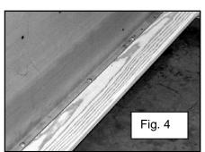
Place a bed strip in the grooves between these boards. The 15. front of the bed strip has a hole at 1-7/8" approximately. Holes in the bed strip should line up with the cross sills and the rear sill. See figure 5. If using MAR-K's custom bed strips with hidden fasteners, follow the instructions supplied with the bed strips for correct installation.
