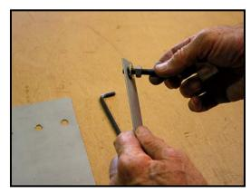
6. Thread the insert onto the bolt with its' flange toward the bolt head. Thread it all the way until finger tight against the scrap metal piece installed in step #5.
