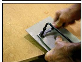
9. The insert will bulge out around its sides causing the insert to clamp down around the hole. Make sure to keep this assembly tight against the panel until the insert is fully squeezed and locked in place. The hex nut will be fairly hard to turn, so be prepared to exert some force on the nut. Turn the nut until it will not turn any more and the insert will be fully installed. Now remove the bolt, hex nut, washer, and sheet metal handle.
