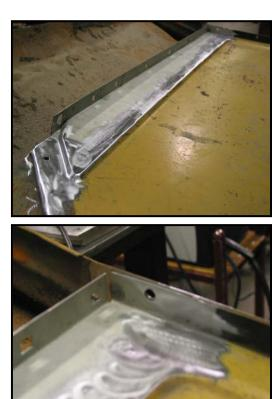
13. The rear section is installed in the same way except it does not have a bent flange at the rear where it meets the bedside rear stake pocket. This panel rests on top of the rear stake pocket and is spot welded a couple of times. Use the same measurement method to locate the panel and also check the fit with the wheel house as before.
