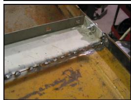
11. We need to re-create the two spot welds at the front panel flange that were drilled out. You will need to remove the paint around these holes also as shown Clamp these panels together and weld through the holes that were drilled to remove the original panel. You may use an aluminum block or copper to back up the panel so that you do not burn through the repair panel with the plug weld.
