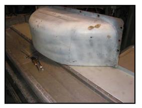
20. Be patient with this part of the process. Skip around from the rear to the front removing one screw at a time and plug welding that hole. You do not want to build up too much heat and warp anything.
