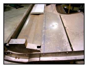
2. Using a jigsaw or other suitable cutting device saw along this line towards the front of the bedside. Use a short blade on the saw to avoid hitting the outer bedside skin. Try to stay on the scrap side of the line away from the bedside spot weld seam.
