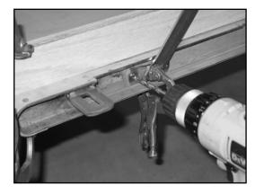
14. Remove the clamps securing the link to the tailgate and remove the link assembly from each end of the tailgate. Use a 1/4" drill to drill holes in the tailgate end that were marked in step 13 above. These holes are exactly 2-1/16 inches apart. Deburr the holes.
