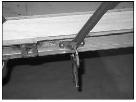
12. Mount the pivot bracket against the sheet metal angled brace spot-welded inside the tailgate end. The pivot bracket should be parallel to the tailgate end. Do this on both ends of the tailgate. Both link assemblies should now be clamped in the position they will be installed on the tailgate end.
