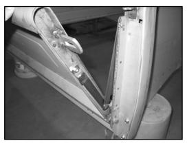
This completes the installation of the check link straps. The tailgate may now be removed to detail and paint the areas cut away. When assembling the system for the final time, use thread locking compound to help prevent the screws from coming loose.
