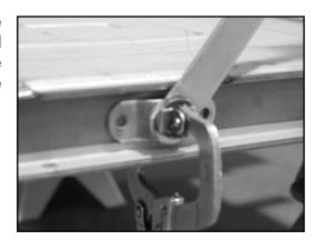
13. Using a 1/4" drill, drill through the holes of the pivot bracket into the tailgate end. Do not drill through, but drill deep enough to effectively mark the hole locations on the tailgate end. Use care to keep the drill square so that the holes in the pivot bracket are not damaged by the drill.
