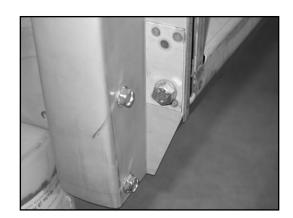
3. Remove the tailgate and the trunnions from both bedsides. Use the template provided to locate the hole for the upper fixed pivot pin for the link straps. Bolt the template to the trunnion hole on the inside of one bedside with the hardware provided. Place the two washers between the template and the bedside. The notched side of the template should be facing the bedside. Mark the bedside through the templates upper hole.
