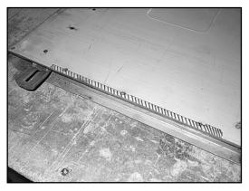
7. Cut away the marked area as measured in Step 6. Use a cutoff wheel or a jig saw with a short blade. Use care at the upper part of the cut to prevent damaging the tailgate latch ear.
