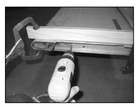
15. Install the link assembly on each end of the tailgate. Use the 1/4" button head screws through the holes drilled in step 14 above to attach the pivot brackets to the tailgate ends. Tighten the screws. If you are installing Mar-K's stainless link assemblies, you must place the button head screws on the side of the tailgate end with the pivot bracket of the link assembly.
