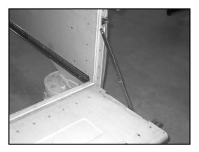
If a full tailgate cover is to be used, weld the bolts holding the link assembly to the tailgate ends in place. This will allow you to still remove the link assemblies if needed after the full tailgate cover has been installed.
