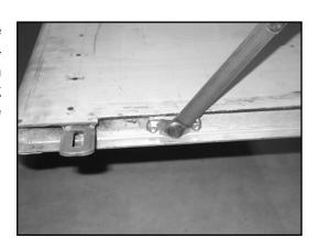
16. Remove the board used to hold the tailgate parallel to the bed floor in step 10 above. Carefully raise the tailgate to the closed position. The links should fold smoothly into the tailgate end as the tailgate is raised. The tailgate should move to the fully closed position without causing any binding in the link assembly.
