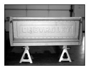
2. Install the trunnions and tailgate and make sure it is aligned to your satisfaction. The trunnion bolt hole in the bottom of the bedsides is slotted to allow adjustment of the tailgate to the bedsides. The tailgate should be adjusted to be nearly touching the rear sill when closed but no more than 1/32" gap. Check the operation of the tailgate. Make sure it operates freely without binding.
