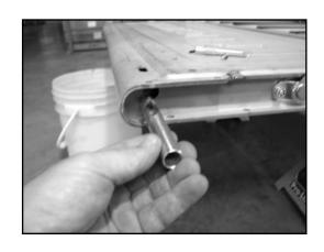
11. Thread the 10-32 button-head screw through the tailgate into the latch sleeve and tighten with the supplied 1/8" hex wrench. Check the alignment of the slot in the tailgate with the slot in the latch sleeve.
