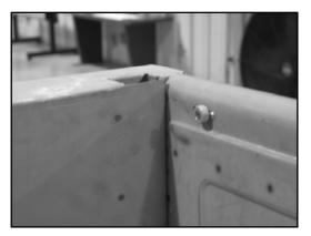
15. Lower the tailgate and support it in the open position. At each marked location on the bedsides, you need to drill a 5/8" diameter hole. It is better to start with a small drill and work up to the 5/8" diameter to ensure a more uniform round hole.
