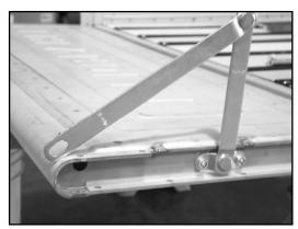
8. Raise the tailgate assembly while folding the link assemblies upward. Align the slot in the link assembly to the flat sides of the pivot pin and slide the link onto the pivot pin. Lower the tailgate back to the open position while letting the link assemblies support the tailgate.
