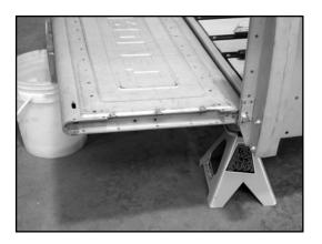
7. Bolt the link assemblies to the tailgate ends using the supplied 1/4-20 x 1/2" button head screws and 1/4" lock nuts. Place the nuts on the same side of the tailgate ends with the links. This will make only the button heads visible when the tailgate is shut.
