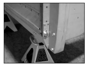
3. Remove the tailgate and the trunnions from both bedsides. Use the template provided to locate the hole for the upper fixed pivot pin for the link straps. Bolt the template to the trunnion hole on the inside of one bedside with the hardware provided. Place the two washers between the template and the bedside. The notched side of the template should be facing the bedside. Mark the bedside through the templates upper hole.
