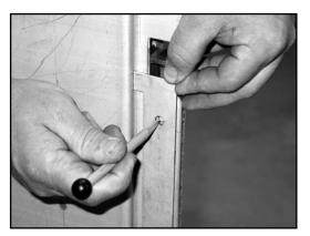
4. Remove the template and center-punch this location. Drill a 5/16" hole through the bedside at that location. Do this for both bedsides and debur the drilled holes.
