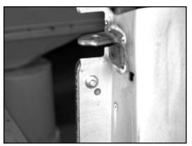
6. Re-install the tailgate and align it as before. Open the tailgate and support it so that it is in the horizontal position.
