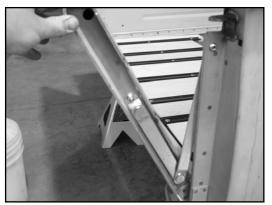
10. Lower the tailgate down to the open position again. Next you need to install the hidden latch barrels into the tailgate ends. It does not matter which one goes into which end of the tailgate at this time. Slide the latch sleeve into the tailgate through the 5/8" hole until the small threaded hole lines up with the small hole in the tailgate.
