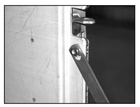
Carefully raise the tailgate to the closed position. The links should fold smoothly downward and then into the tailgate end as the tailgate is raised. The tailgate should move to the fully closed position without causing any binding in the link assembly.
