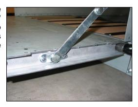
10. Carefully raise the tailgate while folding the links in the upward direction. This will allow the slot in the link assembly to fit onto the fixed pivot that you bolted to the bed side.
