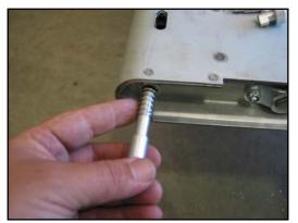
15. Place the shoulder bolt through the knurled side of the aluminum knob. Push in on the plunger until the threaded area of the latch plunger is visible in the slot. Thread the shoulder bolt into the latch plunger. Tighten the bolt with the supplied hex wrench.
