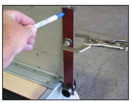
6. Center punch these locations and drill a 5/16" hole through the bedside. Do this for both bedsides and deburr the drilled holes.
