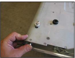
16. Pull the knob towards the center of the tailgate and twist to lock it into position. You may need to twist up or down depending on which latch barrel and plunger you put in. You may also switch these from end to end on the tailgate to reverse this direction.
