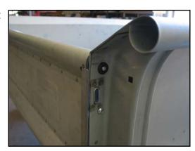
You have now successfully installed your new tailgate, hidden latch system, and the link assemblies. During final assembly, use a quality lubricant on all the moving parts and a thread locking compound on the assembly hardware.
