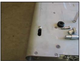
14. The latch plunger and the latch barrel need to match. The latch plunger and the barrel have an angled cut on them that controls the direction of the locking knob. The angle on these needs to be pointing the same direction as shown. Slide a spring onto the latch plunger and slide the assembly into the latch barrel.
