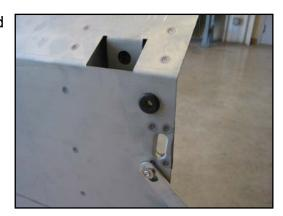
20. Close the tailgate and release both latches. Make sure that they enter the grommets.
