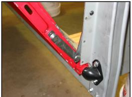
18. This completes the installation of the check link straps. The tailgate may now be removed to detail and paint the areas cut away. When assembling the system for the final time, use thread locking compound to help prevent the screws from coming loose.
