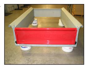
3. Mark the location of one hinge so it may be removed and reinstalled in the exact same location. This may be done by scribing around the hinge, using masking tape to outline the hinge, or placing masking tape on the mounting surface before installing the hinge and then drawing an outline on the tape with a pencil or pen.
