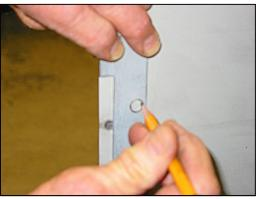
6. Center punch this location and drill a 5/16" hole through the bedside at that location. Do this for both bedsides and deburr the drilled holes.
