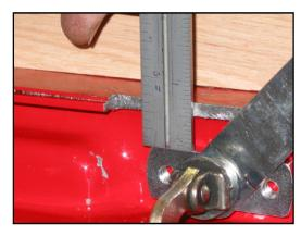
14. Using a 3/16" drill, drill through the holes of the pivot bracket into the tailgate end. Do not drill through, but drill deep enough to effectively mark the hole locations on the tailgate end. Use care to keep the drill square so that the hole in the pivot bracket is not damaged by the drill.
