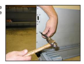
7. Install the fixed pivot pin at each of the 5/16 holes drilled in step 6 above. Use the 5/16" diameter button head screw to attach each pivot pin. The screw head is on the outside of the bedside and the fixed pivot pin is on the inside of the bedside. Place the stainless washer over the fixed pivot pin before bolting it to the bedside. Tighten the fixed pivot pin so that its flat edges are horizontal as shown in the photo.
