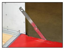
17. Remove the board used to hold the tailgate parallel to the bed floor in step 12 above. Carefully raise the tailgate to the closed position. The links should fold smoothly into the tailgate end as the tailgate is raised. The tailgate should move to the fully closed position without causing any binding in the link assembly.
