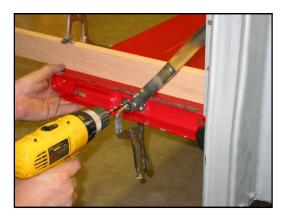
15. Remove the clamps securing the link to the tailgate and remove the link assembly from each end of the tailgate. Use a 1/4" drill to drill holes in the tailgate end that were marked in step 14 above. These holes are exactly 1-1/2 inches apart. Deburr the holes.
