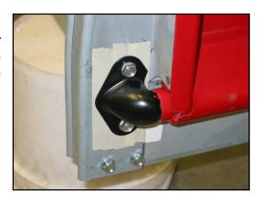
4. Remove the hinge that was marked in step 3 above, and remove the tailgate. Install the hinge back in the same location so that both hinges are in the exact mounting position they were when the tailgate was installed and properly aligned
