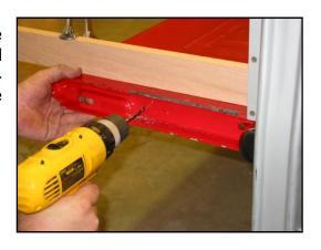
16. Install the link assembly on each end of the tailgate. Use the 1/4" button head screws and locknuts through the holes drilled in step 15 above to attach the pivot brackets to the tailgate ends. The screw head must be on the pivot bracket side. Tighten the screws.
