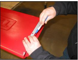
9. Cut away the marked area as measured in Step 8 above. Use a cutoff wheel or a jig saw with a short blade. Use care at the upper part of the cut to prevent damaging the tailgate end.
