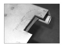
9. Attach the template to the bedside again. Fit the patch panel to the template. The patch has a hole pattern that matches the template. Check the fit or gap around the patch to the bedside. Clamp the template and patch to the bedside. Make sure that the patch and template stay even with the back edge of the bedside. You may use the bolts and 5/16" nuts provided if you wish to bolt the patch to the template.
