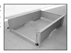
2. Attach one tailgate hinge to the right or left rear stake pocket with two 5/16-18 x 3/4" hex head bolts. Leave them loose for now. Slide the tailgate lower hinge tube onto the hinge on the stake pocket. Insert the other hinge into the opposite hinge tube of the tailgate. Attach it to the stake pocket as before.
