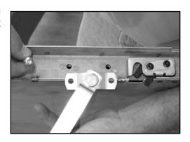
5. Attach one tailgate hinge to the right or left rear stake pocket with two 5/16-18 x 3/4" hex head bolts. Leave them loose for now. Slide the tailgate lower hinge tube onto the hinge on the stake pocket. Insert the other hinge into the opposite hinge tube of the tailgate. Attach it to the stake pocket as before.
