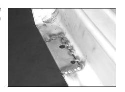
12. Grind all welds smooth. Again, be careful not to build up too much heat with the grinder.
