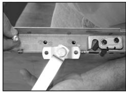
Your new tailgate is supplied with the tailgate latch mechanisms that must be installed. However, before painting you will want to remove these items.
