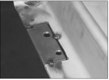
Note: You may wish to re-assemble the box at this point to verify the positions of the patches before permanently welding them in place.
