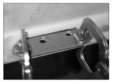
10. Tack-weld the patch into place from the outside of the bedside. Check to see that the patch has not shifted. Remove the template and tack weld from the other side. Do these steps to both bedsides.
