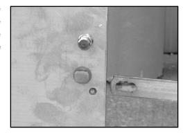
7. Once both check straps are placed on the pins, lower the tailgate to its full open position. Gently close the tailgate while watching the check straps. They should fold together towards the bedsides in a downward motion. Continue closing the tailgate. If any binding occurs, you may need to adjust a hinge up or down. If everything is good then close the tailgate against the strikers. Make sure the handle has been released to open the latches before doing this.
