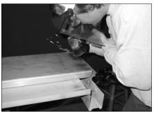
Note: The patch and the bedside should now appear to be the same metal and be smooth at the weld seam.
