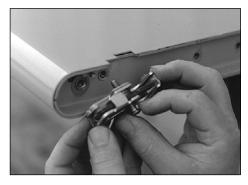
4. Install the check straps to each end of the tailgate using two 1/4-20 x 3/4 " button head torx screws with a T-25 torx driver.
