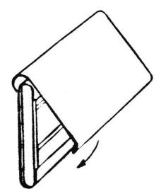
8. Clamp the bottom and sides of the cover to the tailgate, using care not to damage or dent the tailgate cover. Drill 4 holes for pop rivets through the tailgate cover and into the tailgate. Make sure the cover is fully seated onto the tailgate when drilling the 4 holes. Space them approximately as shown. Install pop rivets to secure the bottom of the tailgate cover.
