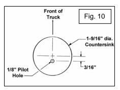
24. Using a 1-9/16" Forstner bit with a 3/8' diameter shank, a drill press if available, or a hand drill, countersink each bed-to-frame location approximately 1/8" to 3/16" deep on each mark from step #23. See figure 11. This offset hole is for the offset washer. The offset washer keeps the bolt from turning.
