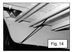
29. Attach rear wheel splash aprons to bed sides. Bolt splash apron to bedside first. Align two holes in splash apron to lower rear leg of cross sill and mark holes through splash apron. Remove splash apron and drill these two holes with a 3/8" drill. Replace splash apron with four bolts. See figure 15.
