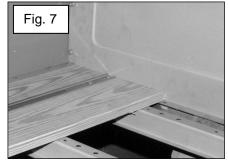
inches from the front of the bed. One reinforcement strip is 72" and one is 49-1/2". Attach these reinforcement strips to the bolts from the bed sides and the wheel well. Mount the 72" at the front of the wheel well and the 49-1/2" reinforcement strip at **48-1/8** inches.
