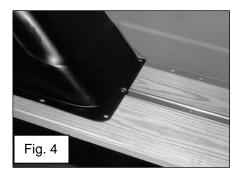
12. Install a 5/16"-18 x 1-1/2" carriage bolt through the wheel well and through the bed strip. Use a 1-1/2" outside diameter flat washer and 5/16" nut to hold the short wood boards to the wheel well. See figure 4.
