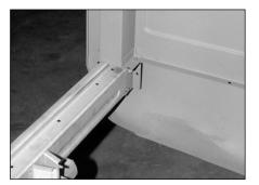
8. Re-install wheel well if removed. The bottom lip of wheel well sits on top of the bedside lower flange. The wheel well is held in place with 5/16"-18 x 3/4" indented hex washer head bolts as needed.
