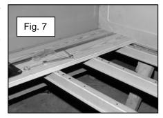
connects to the ninth bed strip hole at **83** inches from the front. There are two smaller cross members located at the front or beginning of the wheel well and at **60-1/8** inches from the front of the bed. One reinforcement strip is 72" and one is 49-1/2". Attach these reinforcement strips to the bolts from the bed sides and the wheel well. Mount the 72" at the front of the wheel well and the 49-1/2" reinforcement strip fits between the wheelhouses at **60-1/8** inches.
