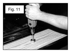
25. To finish this procedure, drill a 1/2" hole through the boards using the pilot holes drilled in step #22 as a guide. See figure 12.
