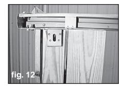
18. The third bed-to-frame bolt location does not pass through a cross sill. There are two brackets attached to the rear cross sill. These large brackets should fit against the bottom of the wood boards.
