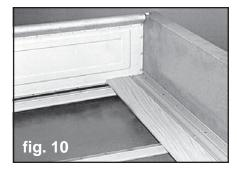
16. The first cross sill at the front is the first bed-to-frame hole location. Mark the bottom of the second boards from each side through the 1/2" diameter cross sill holes that are **36-5/8**" apart from center of hole to center of hole. See figure 11.
